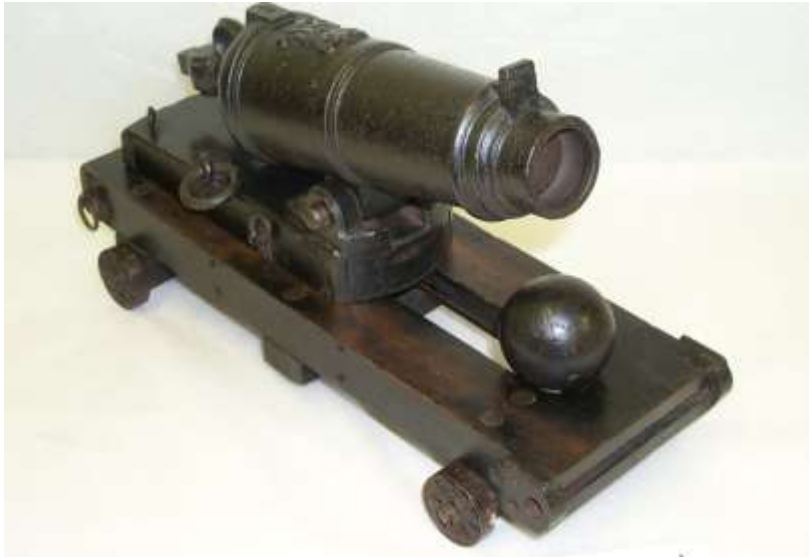
Illus: Model carronade based on GD58/8/85 in the Carron archive, showing the sliding carriage.
